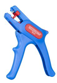
The WEICON Wire Stripper No. 5 is suitable for stripping all stranded and solid conductors from  $0.2 - 6.0 \text{ mm}^2$ . The wire stripper also has a visual length scale from 5 - 12mm. The length stop can be removed, if required. A well-accessible side cutter is integrated in the tool, which is suitable for cable diameters up to 2 mm. The blades are replaceable. The low weight of the No. 5 ensures fatigue-free working.
